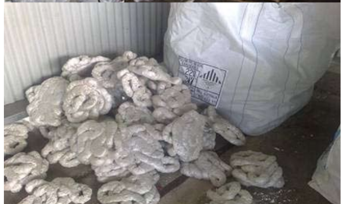
Foam boxes are volume reduced by 90 times to recyclable ingots.
